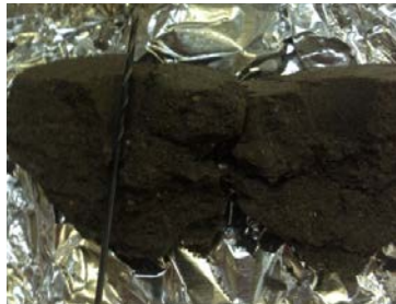
Figure 63. Inner size of hole compared with drill needle for alluvial top stratum
