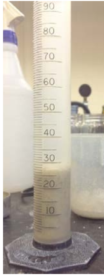
Figure 85. Final swell volume for modified free swell test for treated bentonite
