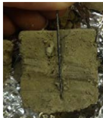
Figure 97. Inner size of hole compared with drill needle for Santa Rosa clay
