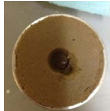
Figure 96. Aerial size of hole after pinhole test completion for Santa Rosa clay
