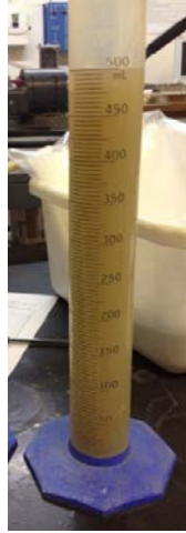
Figure 102. Effluent from pinhole test for sodium illite
