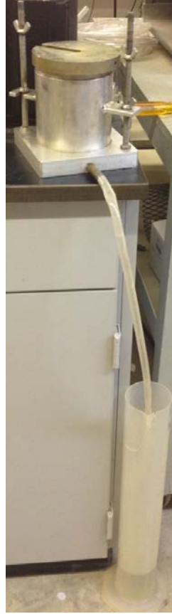
Figure 51. View of compaction permeameter system used to compress sodium illite
