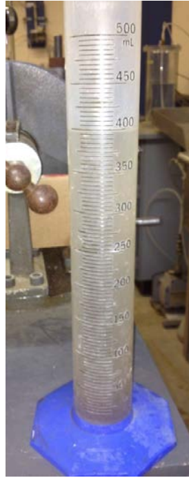
Figure 61. Effluent from pinhole test for alluvial top stratum
