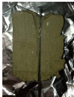
Figure 70. Inner size of hole compared with drill needle for Western Iowa loess
