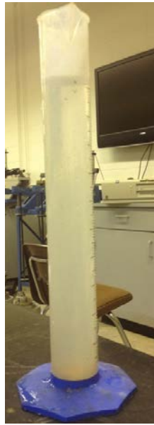
Figure 54. Effluent from pinhole test for oxidized till
